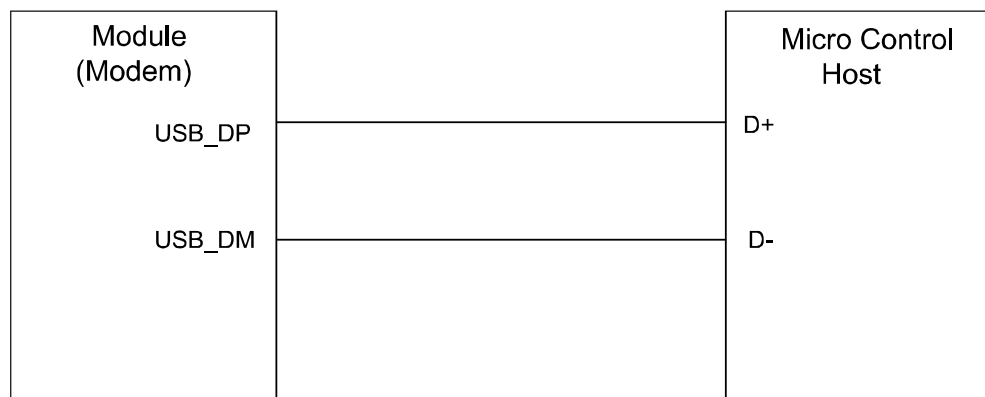
Figure 3-11 Recommended circuit of USB interface
