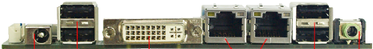
12V DC-IN JACK 2 * USB 2.0/1.1 ports DVI-I port 2 * RJ-45 ports 2 * USB 2.0/1.1 ports Line-out port
