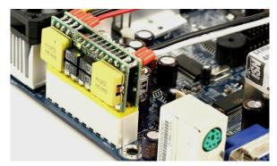
Fig 1.1 picoPSU-150-XT plugged into ATX connector.
